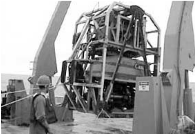
ROPOS being deployed for deep water operations inside its steel cage.
