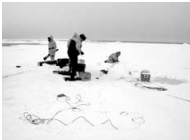
The science team lowers a string of sample bottles through holes drilled in the ice to collect plankton at different water levels. Notice the polar bear observer standing to the left.
