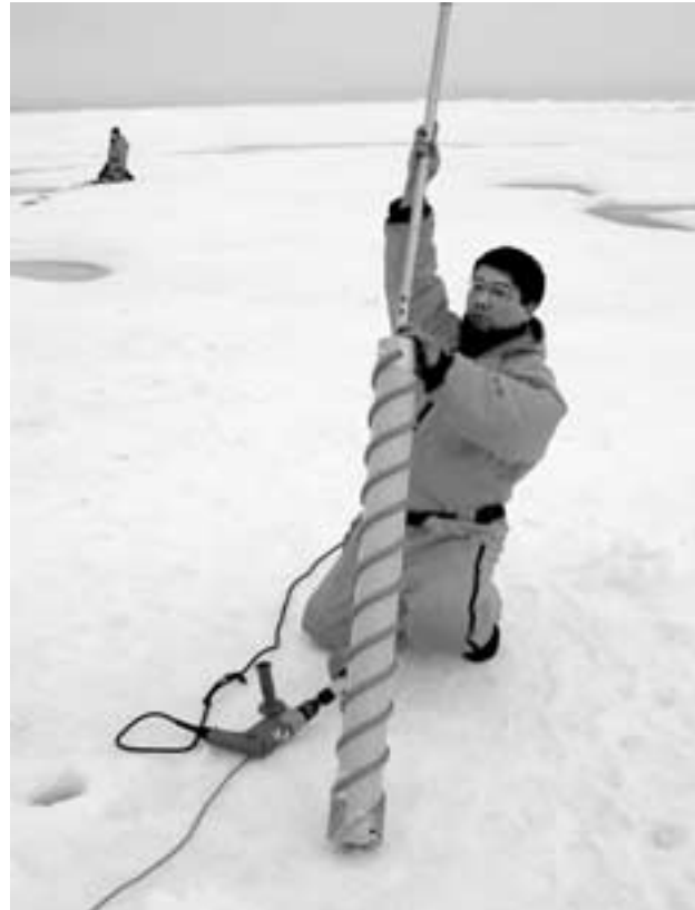
Qing Zhang, a member of the Chinese science team, removes a long cylindrical core of ice from the thick Arctic ice pack.
