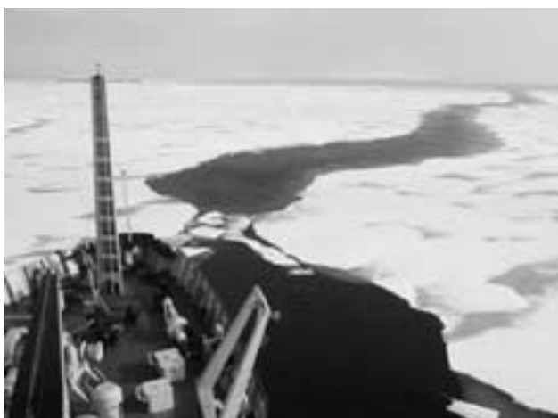
A view from the bow of the Louis St. Laurent shows a lead. Ice leads are cracks in the thick ice cover that vessels use because it minimalizes time spent breaking through the ice.
