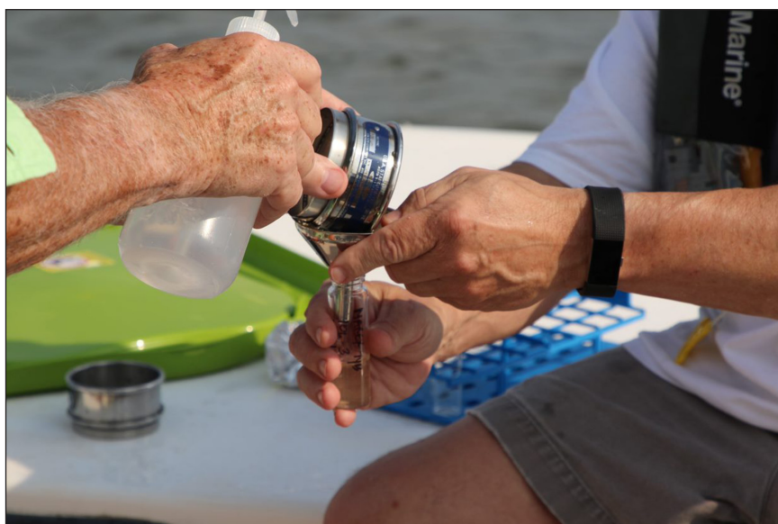
Figure 5: Samples rinsed from stainless steel sieves. Photograph by D. Sanders.
