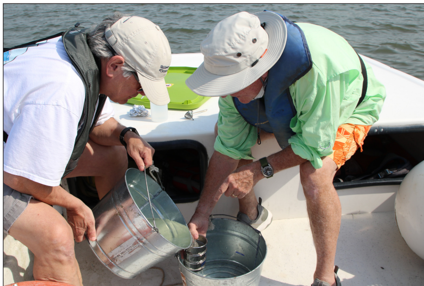
Figure 4: Samples of seawater are poured through a series of stainless steel sieves. Photograph by D. Sanders.
