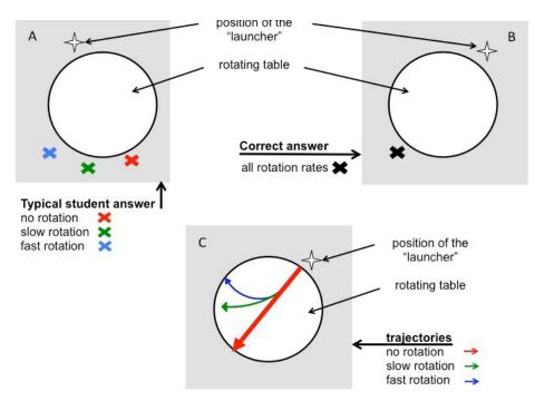
FIGURE 4 (A). Depiction of the typical wrong answer to the question: Where would a marble land on the floor after rolling across a table rotating at different rotation rates? (B). Correct answer to the same question. (C). Correct traces of marbles rolling across a rotating table.
