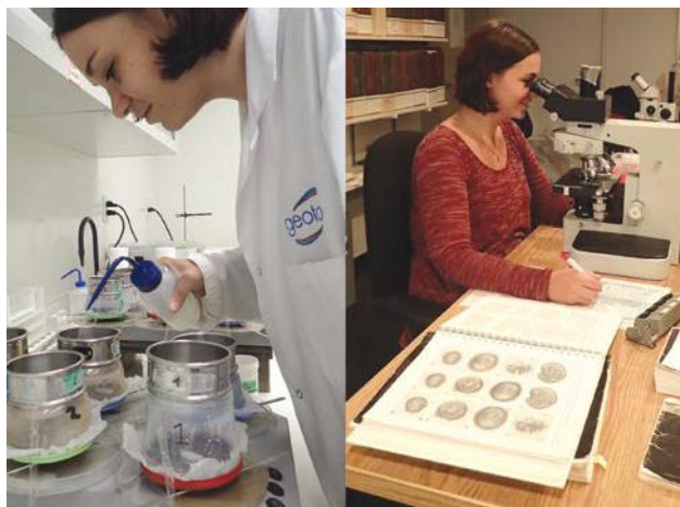
FIGURE 6. Back in the laboratory Estelle washes and sieves the samples to separate the dinocysts from the sediment. Once samples are prepared, Estelle uses her microscope and dinocyst reference catalogues to complete her identification. Courtesy of Jade Falardeau
