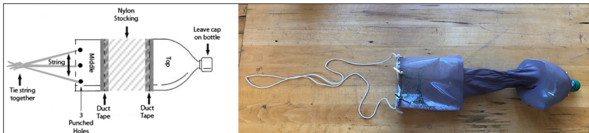
Figure 2: Diagram of how to construct a makeshift plankton tow (left; from NJ Sea Grant Consortium), and a photograph of the assembled phytoplankton tows used by Mr. Hinkel's fifth grade class (right). Photo: Kyla Kelly. Reproduced with permission of the photographer.
