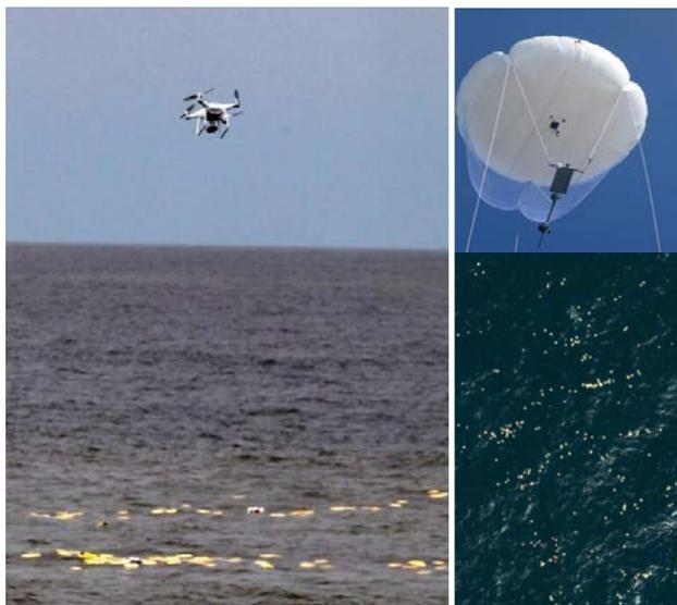
**FIGURE 7.** (left) Drone monitoring a patch of drift cards during an experiment examining the near-surface layer of the ocean; (right top) high-resolution camera system hanging from the aerostat; (right bottom) image from the aerostat camera of thousands of drift cards gathering into lines during a dispersion experiment. Courtesy of CARTHE
